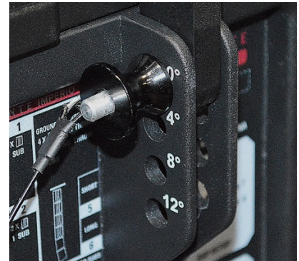
Adjust throw angle by attaching integrated adjustable mounting bracket from Imperio speaker, swinging it down to desired throw angle mounting hole on bottom Imperio speaker or Flybar, secure with Linkpin 2 .
