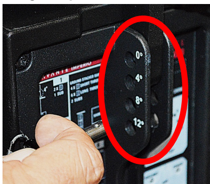
Adjust throw angle by attaching integrated adjustable mounting bracket from Imperio speaker, swinging it down to desired throw angle mounting hole on bottom Imperio speaker or Flybar, secure with Linkpin 2 .
