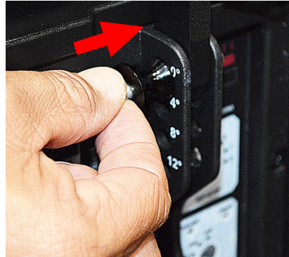
Adjust throw angle by attaching integrated adjustable mounting bracket from Imperio speaker, swinging it down to desired throw angle mounting hole on bottom Imperio speaker or Flybar, secure with Linkpin 2 .
