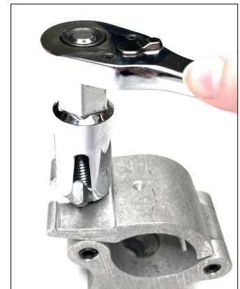
4. Tighten or Loosen - Use the Wing Nut Socket to adjust the wing nut over the screw with ease, with more reliability than possible by hand.
