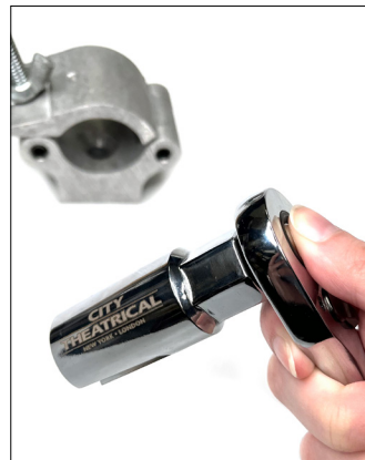
2. Test - Test the fitment of the Wing Nut Socket on the ratchet to ensure a secure fit.
