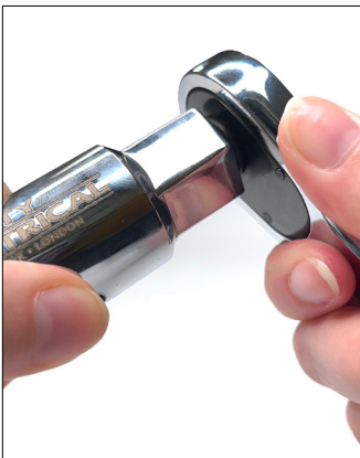
1. Attach - Attach the Wing Nut Socket to a 3/8" ratchet with a push button to secure the socket placement.
