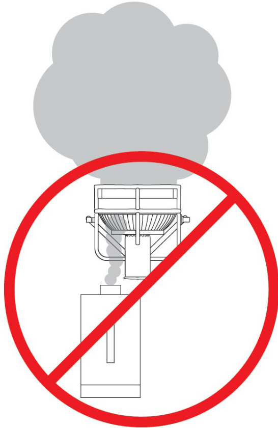
Incorrect ProFan placement in front of fogger/hazer
